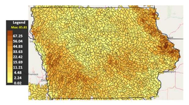
**Figure 3.** As an example, estimated annual soil loss for the 2017–2018 water year across Iowa, illustrating erosion rates from 3 to more than 70 Mg/ha. The latter corresponds to an erosion rate of roughly 6 mm (0.2 inch) of soil loss in four years. Figure courtesy of the Daily Erosion Project (www.dailyerosion.org).
