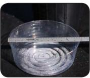
Figure 59. Measure catch can diameter
