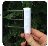
Figure 38. Soil/substrate moisture sensor
