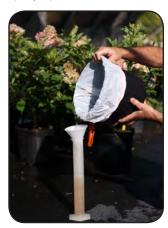
Figure 58. Measure irrigation captured
