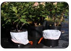
Figure 56. Plant in drainage can and catch can of equal size
